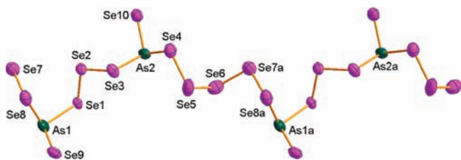
Figure 1. Crystal structure of the helical [\text{As}_2\text{Se}_2(\mu\text{-Se}_3)(\mu\text{-Se}_5)^{2-}]_\infty chain in 1 with the labeling scheme (thermal ellipsoids are drawn at 50% probability).
