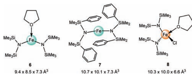
Figure 1. Iron silylamide precursors under study (approximate van der Waals dimensions from crystallographic data are indicated; see also Supporting Information). 70–72
