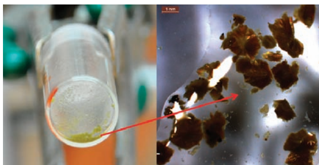
Figure 1. Photographs of crystals of 1 and 2 illuminated by standard room fluorescent lighting (left) and under microscope lighting (right) with a halogen lamp showing the Alexandrite effect.
