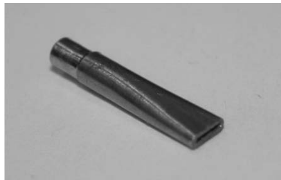
Figure 1. Photograph of an aluminum high-temperature slit nozzle.
