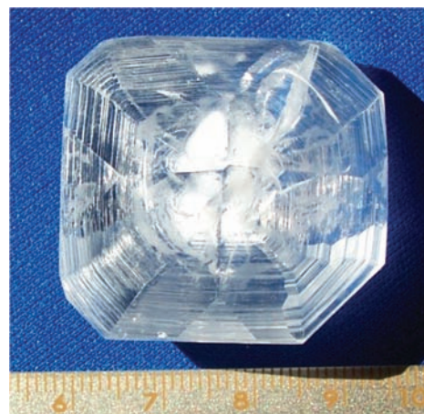
Figure 1. Photograph of NBAC crystal with sizes up to 34 × 34 × 16 mm 3 grown from NaF–LiCl flux.
