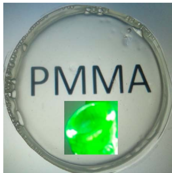
Figure 6. Transparent PMMA film containing a 1 wt % hexagonal \text{KLaF}_4:\text{Er}^{3+} (3 mol %) film. An intense green emission upon shining with white light is shown in the inset.
