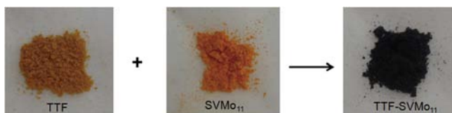
Figure 4. Photographs of TTF, (n-Bu 4 N) 3 [SVMo 11 O 40 ] (SVMo 11 ), and a mixture of TTF and (n-Bu 4 N) 3 [SVMo 11 O 40 ] after grinding together for 1 min (TTF-SVMo 11 ).
