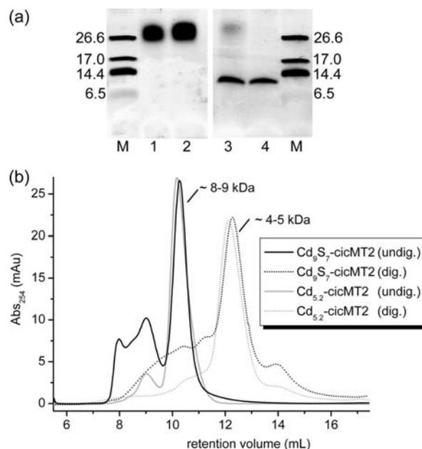
**Figure 2.** (a) Silver-stained SDS-PAGE (12%) of unmodified and mBBR-modified  $Cd_{5.2}$ -cicMT2 (lanes 1 and 4) and  $Cd_9S_7$ -cicMT2 (lanes 2 and 3) relative to a peptide marker (lanes marked with M). (b) Size-exclusion chromatogram of undigested and proteinase K digested  $Cd_9S_7$ -cicMT2 (black solid and dotted lines) and  $Cd_{5.2}$ -cicMT2 (gray solid and dotted lines).
