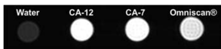
Figure 3. T1-weighted MRI images of CA-12, CA-7, and Omniscan at 1 mM Gd concentration in PBS (25 °C and 7 T).
