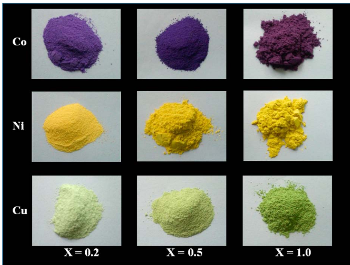
Figure 5. Color of Zn_{2-x}M_xTe_3O_8 oxides for various values of x as seen in the daylight.
