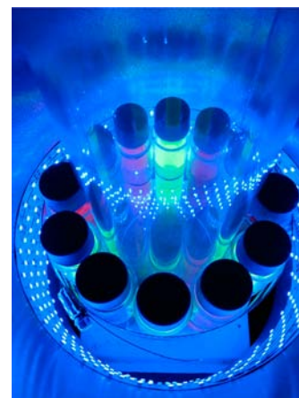
Figure 1. Custom designed photoreactor used in Zn 2+ reducing photoreactions.
