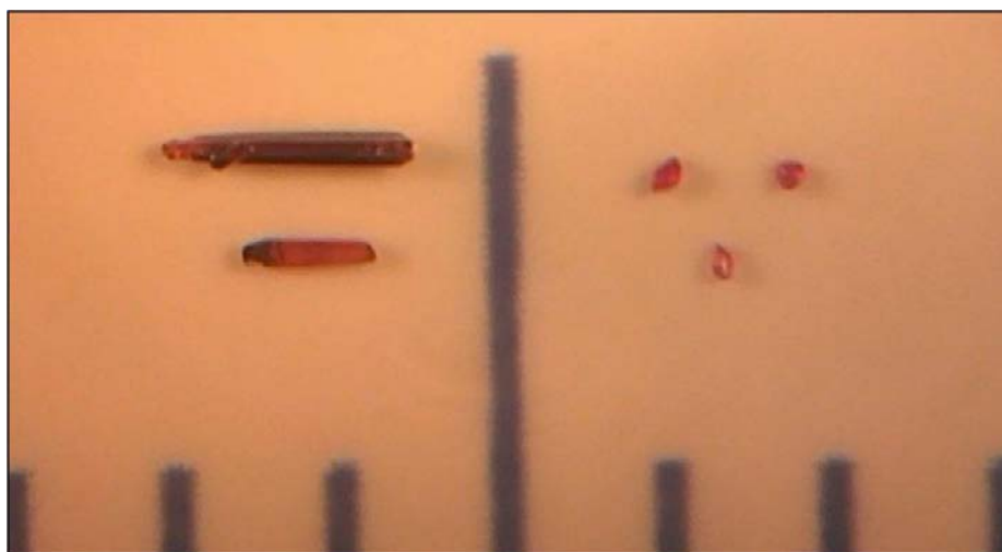
Figure 2. \text{Sr}_2\text{Co}(\text{OH})_6 crystals grown in the presence of a \text{WO}_3 mineralizer (left) exhibiting a different crystal morphology and increased size compared with crystals grown without \text{WO}_3 (right). Graduations are in millimeters.
