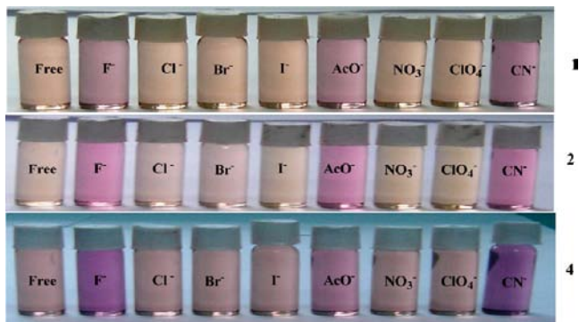
Figure 7. Color changes that occur when the solutions of 1 , 2 , and 4 are treated with various anions as their tetrabutylammonium (TBA) salts.
