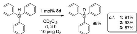
Scheme 3. H/D Exchange on Silanes Catalyzed by 8d
