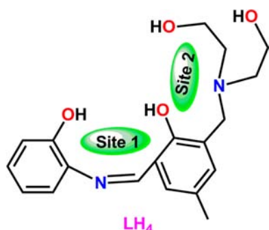
Figure 1. Two distinct coordination compartments of LH_4 . Site 1 contains a chelating ONO coordination manifold while Site 2 provides a scorpionate -like binding cavity.
