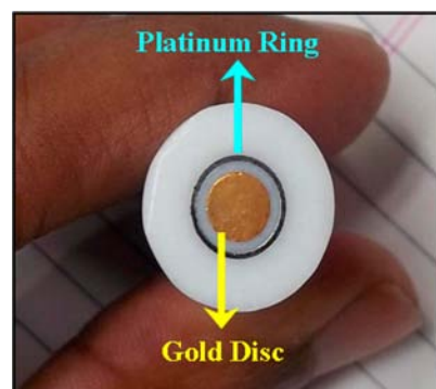
Figure 9. RRDE assembly showing the Au disc and Pt ring.
