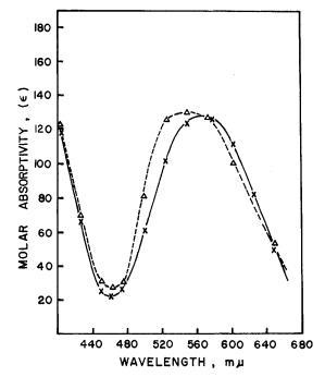
Figure 1.—Visible spectra of cis-[Co(tren)Cl<sub>2</sub>]<sup>+</sup> (×) in 50% HCl and cis-[Co(trien)Cl<sub>2</sub>]<sup>+</sup> ( $\Delta$ ) in 50% HClO<sub>4</sub>.
