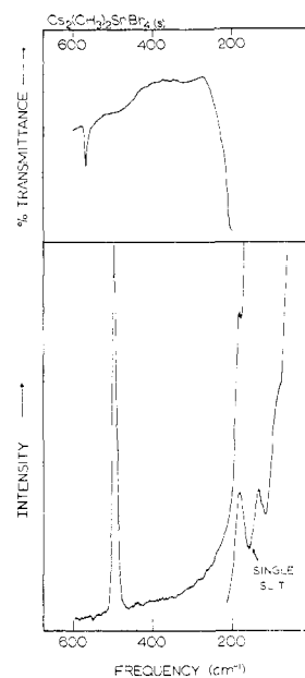
Figure 6.—Infrared and Hg arc excited Raman spectra of Cs_2[(CH_3)_2SnBr_4] in the skeletal vibration region. The signal at ca. 145 cm^{-1} is the grating ghost.
