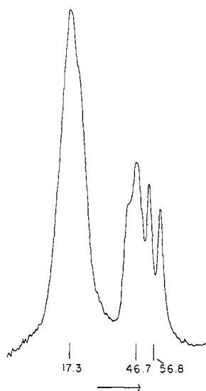
Figure 1.—The 32.1-MHz ^{11}\text{B} nmr spectrum of \text{B}_8\text{H}_{16} .
