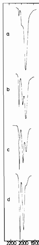
Fig. 1. Changes in the IR carbonyl spectrum of an acetonitrile solution of \text{Fe}(\text{exa})_2 versus time, after exposure to CO for 30 s. (a) 2 min, (b) 5 min, (c) 10 min, (d) 30 min.
