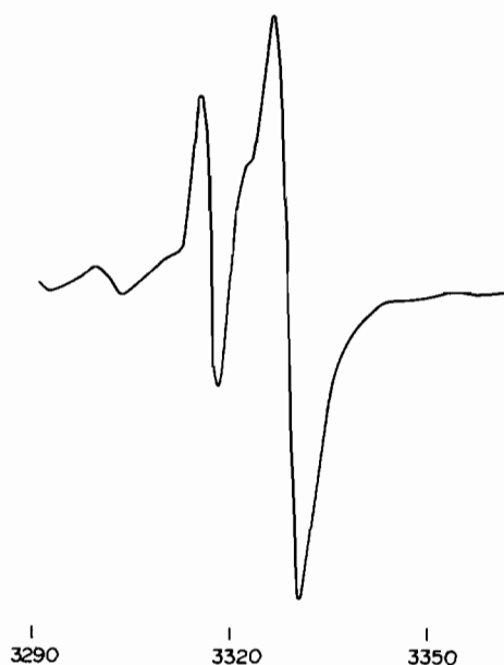
Figure 1c. Esr spectrum of \text{Cp}_2\text{TiPh}_2 for 55 min irradiation in THF at -60^\circ\text{C} and 3 min at -40^\circ\text{C} .
