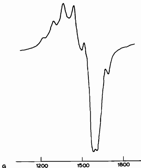
Fig. 7. the e.s.r. spectrum of \text{Cu}_2\text{L}^2(\text{N}_3)(\text{ClO}_4)_3 corresponding to the half-band \Delta M = 2 transition.
