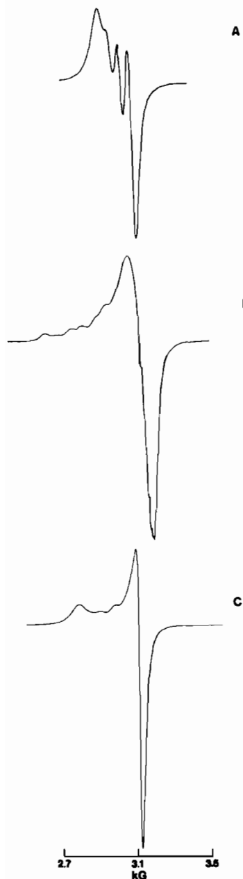
Fig. 1. Representative X-band epr spectra of \text{Cu}(\text{OAc})_2(\gamma\text{-pic})_2 : (A) in \gamma -picoline solution at room temperature, (B) frozen solution at 103 K, and (C) polycrystalline sample at room temperature.
