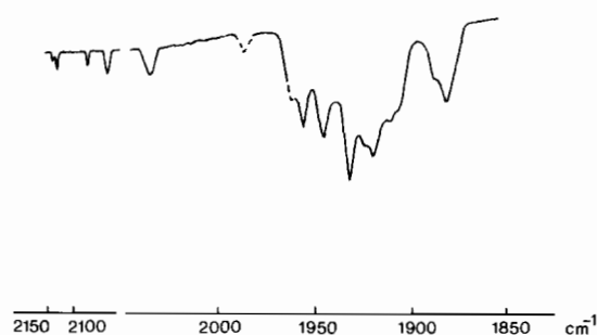
Figure 3. Infrared spectrum of \text{Cr}(\text{CO})_5 pyrazine in an Ar matrix at 10 K after 70 min photolysis with \lambda = 229 nm.
