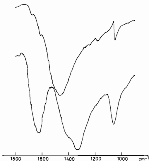
Fig. 2. IR spectra of free (top) and complexed (bottom) ligand in the CO vibration region.
