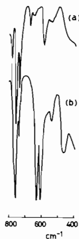
Figure 4. Nujol mull infrared spectra of (a) Mn(SALC 7 ) and (b) Mn(SALC 7 )(O).
