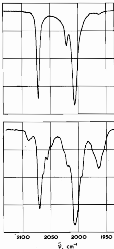
Figure 1. Infrared spectrum of \text{Hg}[\text{Co}(\text{CO})_2]_2 in the C—O stretching region (n-hexane solution) upper trace: with natural abundance of ^{13}\text{C} lower trace: with ^{13}\text{C} content enriched to 22.5 per cent
