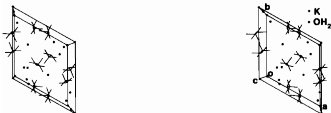
Fig. 2. Stereoscopic view of the packing in the unit cell for K(CH_3)_2N(SO_3) \cdot 0.66H_2O viewed down the c axis.
