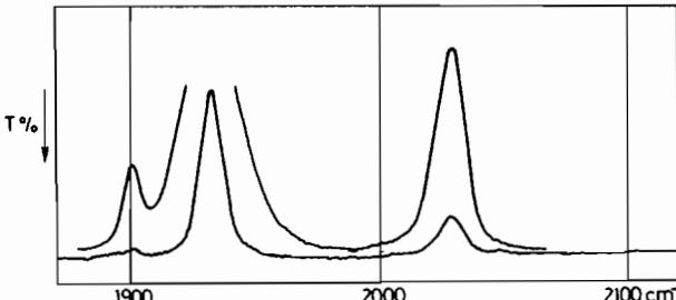
TABLE.  $\nu(\text{C}-\text{O})$  IR Spectra of ( $h^5\text{-C}_5\text{H}_5$ )V(CO)<sub>4</sub> and ( $h^5\text{-AcC}_5\text{H}_4$ )V(CO)<sub>4</sub> (n-hexane solution, LiF prism, UR-20, Carl Zeiss Jena, DCL calibration<sup>20</sup>).
