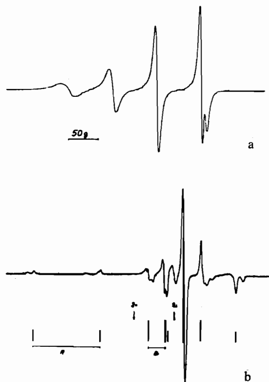
Figure 1. Epr spectrum typical for copper(II) dithiocarbamate complexes in noncoordinating solvent (toluene): a—T=300°K, b—T=77°K.
