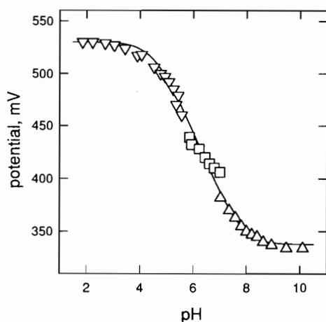
Fig. 1.  $E_{1/2}$  values associated with the oxidation of the ferrocene subunit of the  $\text{FcCOOH}/\text{FcCOO}^-$  system in  $\text{MeCN}/\text{H}_2\text{O}$  solutions (0.8/0.20 vol./vol.), made 0.1 M in  $\text{Bu}_4\text{NClO}_4$ , at 25 °C. The pH was adjusted by using the following buffers:  $\nabla$ , pyridine +  $\text{HClO}_4$ ;  $\square$ , 2,6-dimethylpyridine +  $\text{HClO}_4$ ;  $\triangle$ , ethylenediamine +  $\text{HClO}_4$ .
