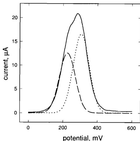
Fig. 4. DPV profile for an unbuffered solution of  $\text{Fc}(\text{CH}_2)_2\text{COOH}$ , of  $\text{pH} \approx 7.7$ . Deconvoluted profiles corresponds to the reversible oxidation of  $\text{Fc}(\text{CH}_2)_2\text{COOH}$  (more anodic peak, centred 305 mV) and of  $\text{Fc}(\text{CH}_2)_2\text{COO}^-$  (less anodic peak, centred at 225 mV).
