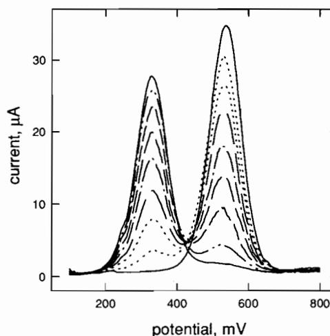
Fig. 2. DPV profiles for unbuffered solutions of  $\text{FcCOOH}$  of varying pH. Increasing the pH makes the peak at 530 mV (corresponding to the oxidation of the  $\text{FcCOOH}$  form) decrease and the peak at 335 mV (oxidation of the  $\text{FcCOO}^-$  form) increase. The pH was varied through the addition of standard base to an acidic solution of  $\text{FcCOOH}$ .
