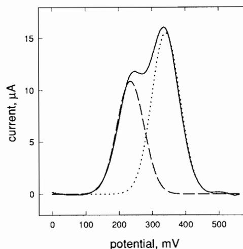
Fig. 3. DPV profile for an *unbuffered* solution of  $FcCH_2COOH$  at  $pH=8.0$  (solid line). The DPV profile has been deconvoluted to give a peak centred at 335 mV (corresponding to the oxidation of the  $FcCH_2COOH$  form) and a peak centred at 220 mV (corresponding to the oxidation of the  $FcCH_2COO^-$  form).
