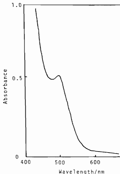
Fig. 2. Absorption spectrum of [\text{Fe}_2\text{O}(\text{CH}_3\text{COO})(\text{L}^3)_2]\text{ClO}_4 (in acetonitrile, 1 \times 10^{-4} \text{ mol dm}^{-3} at 293 K).
