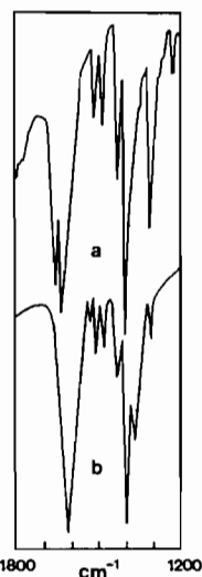
Fig. 2. IR spectra (1800–1200 cm -1 region) of powdered solid samples spread on NaCl disks. (a) [(phen)(Ph 3 P)Cu(O 2 COH)] ( A ); (b) [(phen)(Ph 3 P)Cu(O 2 COH)] ( 3 ).
