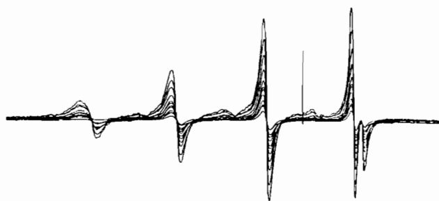
Fig. 2. EPR spectra taken after consecutive 15 min irradiations of the Cu(dtc) 2 complex in toluene.
