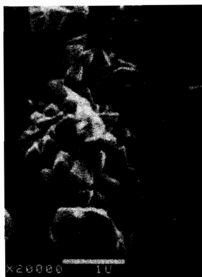
Fig. 2. Scanning electron micrograph of cadmium sulfide powder from the reaction of \text{Cd}(\text{CH}_2\text{SiMe}_3)_2 and \text{H}_2\text{S} .
