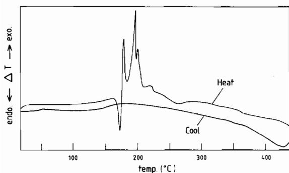
Fig. 2. DTA thermal analysis curves for A, heating rate 20 °C  $\text{min}^{-1}$  in air.
