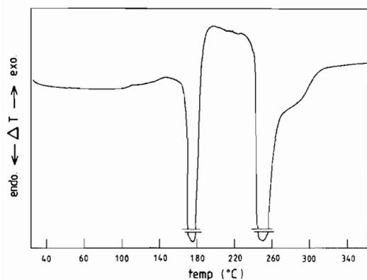
Fig. 3. DTA thermal analysis curve for ferrocene.
