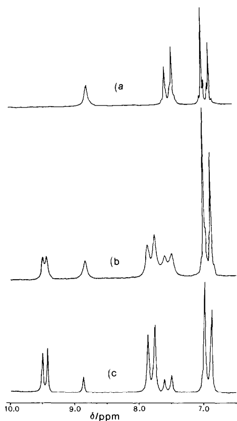
Fig. 3. Variable-temperature ^1\text{H} NMR spectra of 5 \times 10^{-2} mol \text{dm}^{-3} solution of [\{\text{PdCl}(\eta^3\text{-}2\text{-MeC}_3\text{H}_4)\}_2(\text{DAB})] in \text{CD}_2\text{Cl}_2 in the range 10.0–6.5 ppm: (a) 30^\circ\text{C} ; (b) -25^\circ\text{C} ; (c) -50^\circ\text{C} .
