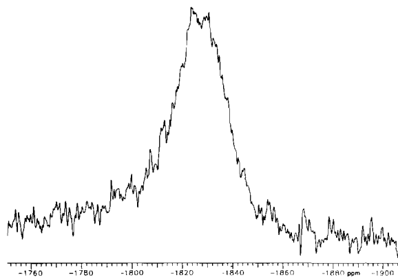
Fig. 2. The ^{99}\text{Tc} NMR spectrum of [\text{Tc}(\text{CN}^t\text{Bu})_5(\text{PPh}_3)]\text{PF}_6 which shows slight splitting due to ^{99}\text{Tc} - ^{31}\text{P} coupling effects.
