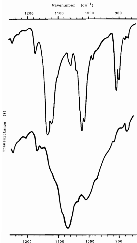
Fig. 5. The IR 1250–850 \text{cm}^{-1} (nujol/NaCl) for [\text{Co}(\text{CNC}_6\text{H}_3\text{Et}_2-2,6)_4(\text{ClO}_4)_2] (top) and [\text{Co}(\text{CNC}_6\text{H}_3\text{Et}_2-2,6)_5](\text{BF}_4)_2 \cdot \text{H}_2\text{O} (bottom).
