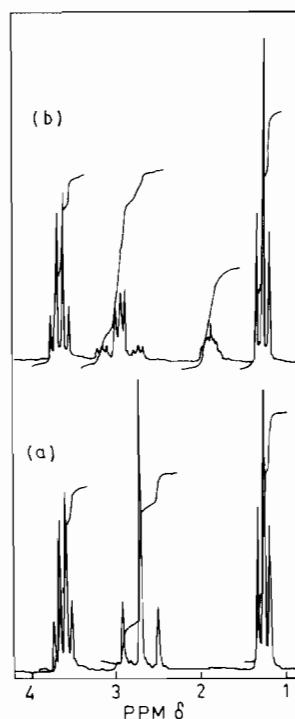
Fig. 1. The 100 MHz ^1\text{H} NMR spectra of (a) [\text{Pt}(\text{en})(\text{DDTC})]\text{NO}_3 , and (b) [\text{Pt}(\text{pn})(\text{DDTC})]\text{NO}_3 , in \text{D}_2\text{O} .
