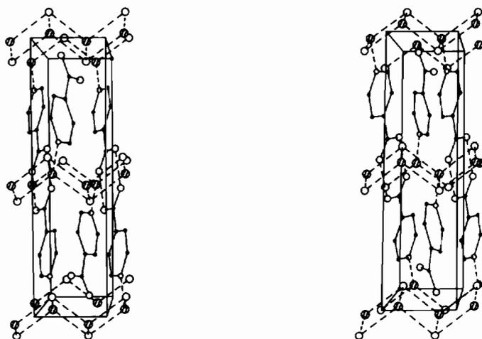
Fig. 2. Stereodrawing of the crystal structure, with metal—ligand bonds represented by broken lines. The unit-cell origin lies at the lower left corner, with *a* pointing towards the reader, *b* from left to right, and *c* upwards.
