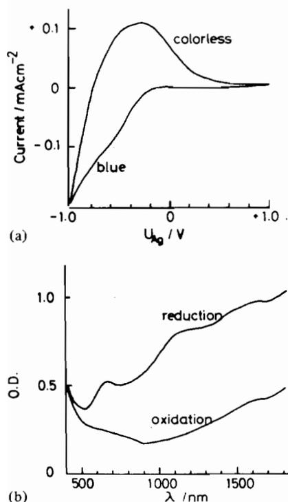
Fig. 3. (a) Cyclic voltammogram and (b) absorption spectra of a  $\text{K}_{0.33}\text{WO}_{3.165}$  ( $d \approx 10 \mu\text{m}$ )-modified ITO electrode.
