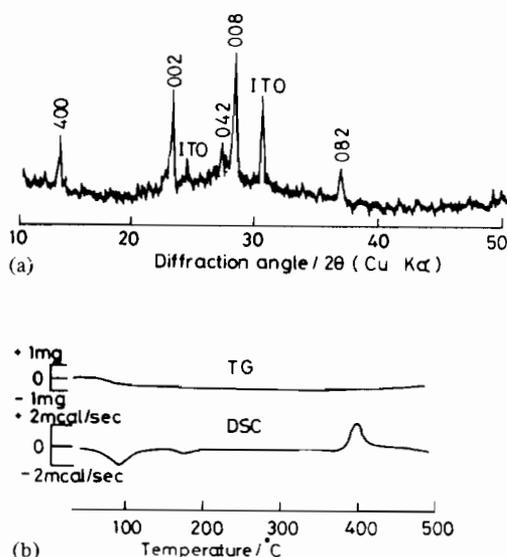
Fig. 2. (a) X-ray diffraction pattern of  $\text{K}_{0.33}\text{WO}_{3.165}$  and (b) thermogram (TG and DSC) curves of the decatungstate deposited cathodically.
