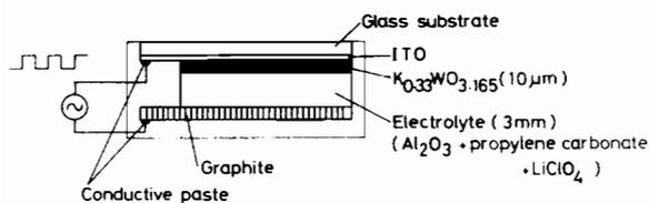
Fig. 5. Schematic configuration (in cross-section) of  $K_{0.33}WO_{3.165}$ -based electrochromic device.
