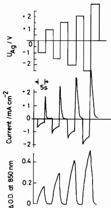
Fig. 4. Cycling characteristics of  $\text{K}_{0.33}\text{WO}_{3.165}$  ( $d \approx 10 \mu\text{m}$ )-modified ITO electrode.
