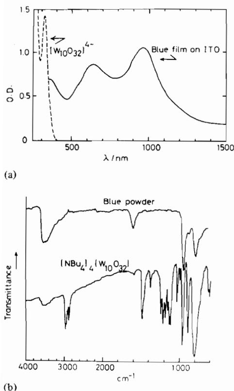
Fig. 1. (a) Electronic absorption and (b) IR spectra for the blue film and  $[\text{NBu}_4]_4[\text{W}_{10}\text{O}_{32}]$ . The two curves in (a) are obtained with the blue film ( $17 \text{ mC cm}^{-2}$ ) deposited on the ITO electrode and the solution (10 mm thickness) containing  $0.1 \text{ mM } [\text{NBu}_4]_4[\text{W}_{10}\text{O}_{32}]$  and  $10 \text{ mM KClO}_4$  in  $\text{CH}_3\text{CN}$ , respectively.
