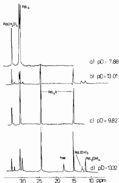
Fig. 5. ^{31}\text{P} NMR spectra of Pd(II):racemic PhGlyP (a, b) and Pd(II):(-)-PhGlyP (c, d) 1:2 solutions.
