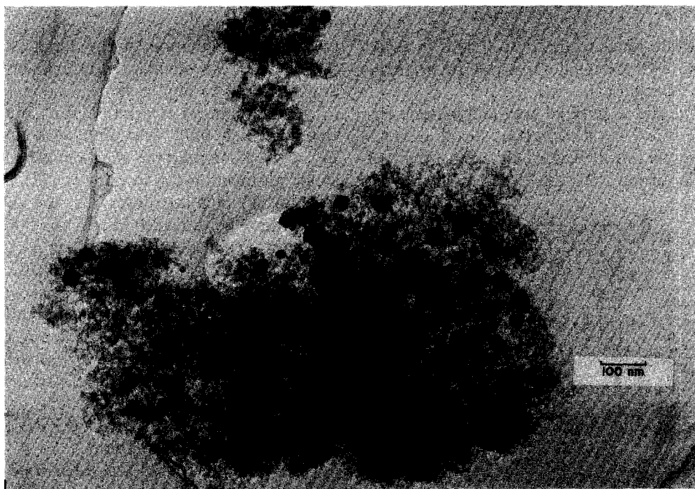
FIG. 5. Transmission electron micrograph of (initially) 5 wt% nickel-catalyzed Sphero carb after pretreatment and steam gasification at 813 K for 60 min.
