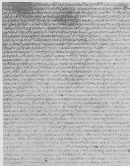
Figure 3. Electron micrograph of a copper phthalocyanine crystal at a magnification of almost 2,000,000 times showing the layer-lattice spacing of 12.5Å. between layers
