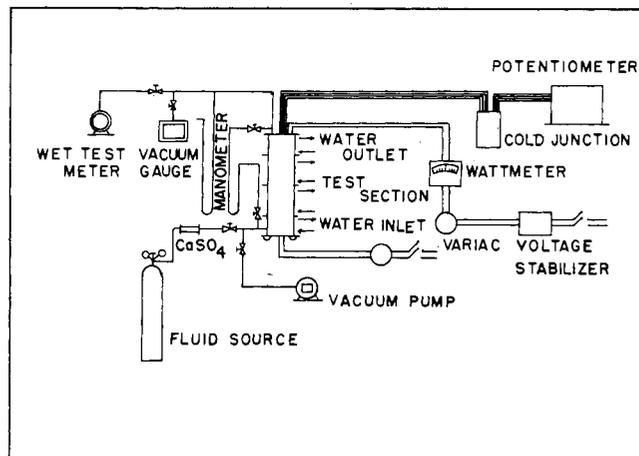
Figure 1. Experimental heat transfer apparatus
