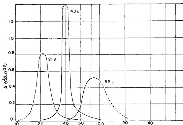
Figure 3. Pore size distribution for Alundum sample
