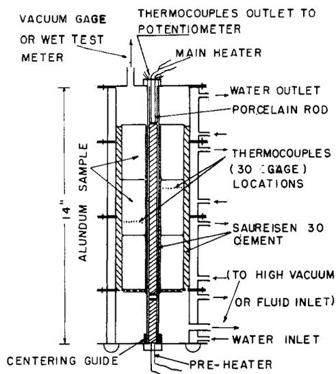
Figure 2. Test section detail
