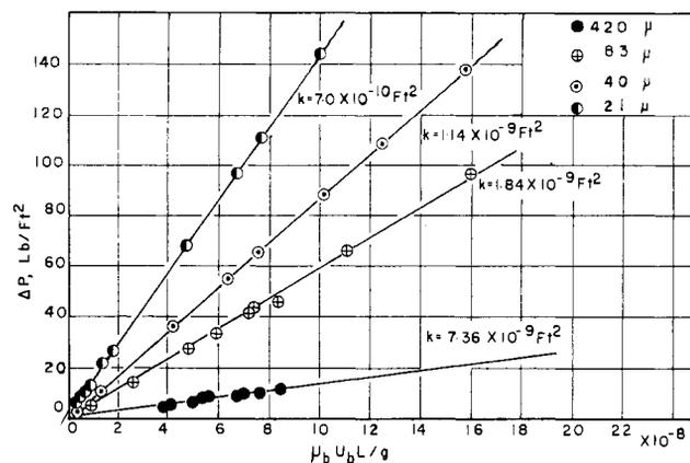
Figure 4. Permeability of Alundum samples (Nitrogen at 21° C.)
