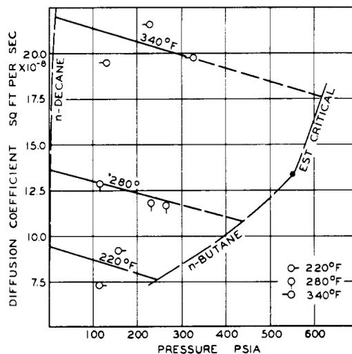
Figure 3. Influence of pressure on Chapman-Cowling diffusion coefficient
