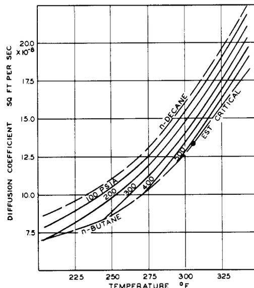
Figure 4. Effect of temperature on Chapman-Cowling diffusion coefficient
