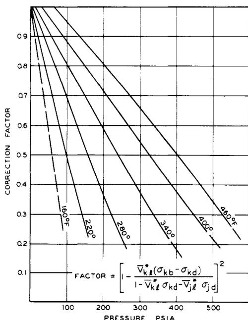
Figure 1. Correction factor for the *n*-butane-*n*-decane system
