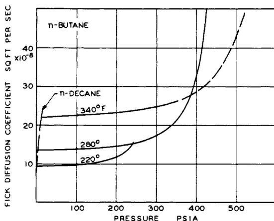
Figure 5. Influence of pressure on Fick diffusion coefficient for *n*-butane
