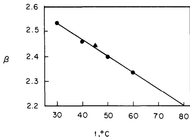
Figure 1. Relative volatility as a function of temperature
