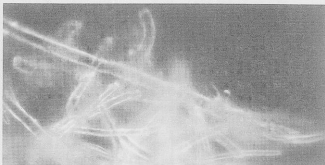
Figure 1. Photomicrograph of fibrous silica surface Fibers are 3.3 to 6 microns in diameter
