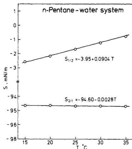
Figure 3. Temperature dependence of spreading coefficients in the *n*-pentane-water system.
