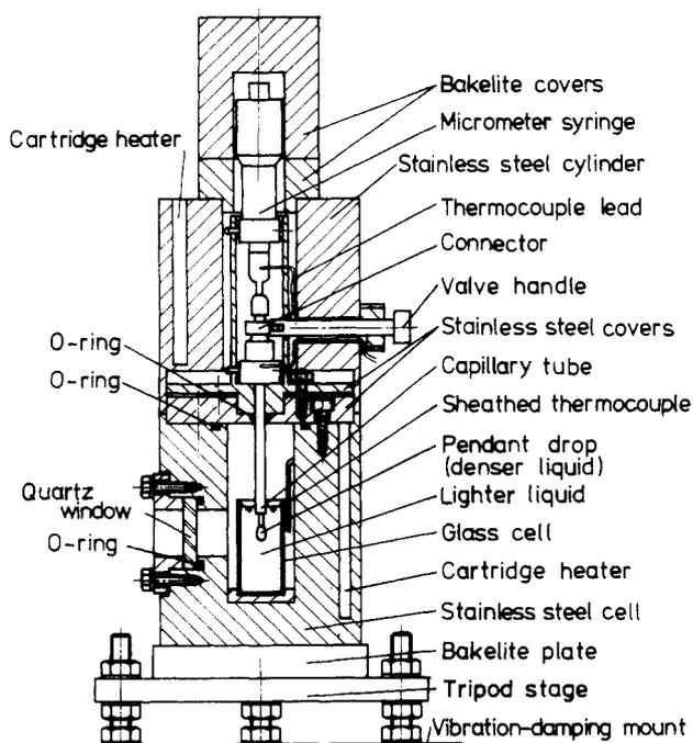
**Figure 1.** Construction of the pendant-drop cell and syringe assembly for liquid-liquid interfacial tension measurement.
