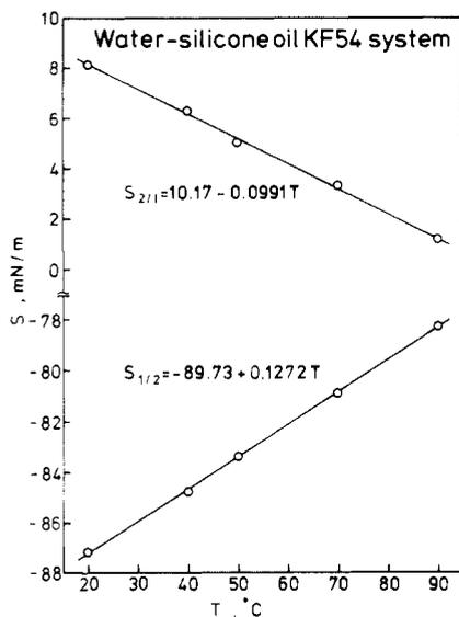
**Figure 5.** Temperature dependence of spreading coefficients in the water-silicone oil KF 54 system.
