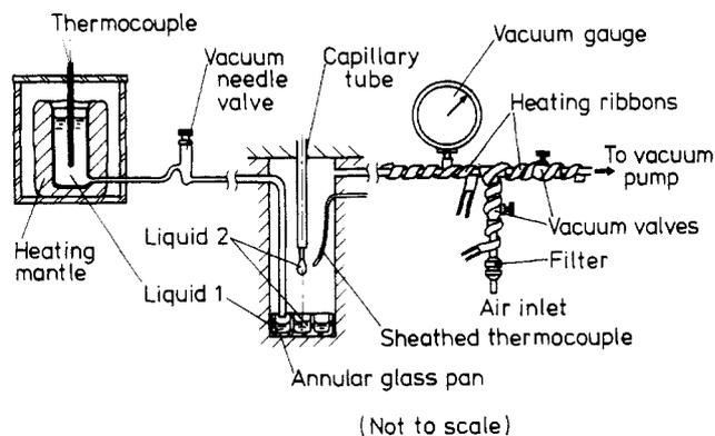
**Figure 2.** Setup of the pendant-drop cell and the auxiliary equipment for surface tension measurement.
