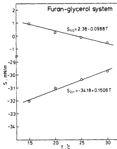
Figure 4. Temperature dependence of spreading coefficients in the furan-glycerol system.
